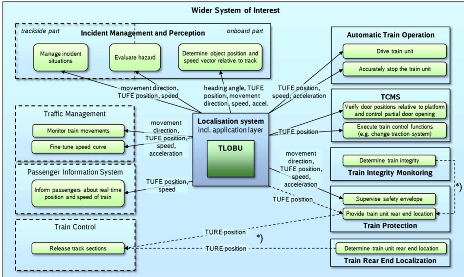
\*) Depending on their type, some trains will determine their rear end indirectly with help of train integrity monitoring and others by a dedicated rear end localization system. The exact distribution of functions for this purpose is outside the scope of CLUG. (see 2.1.5)
