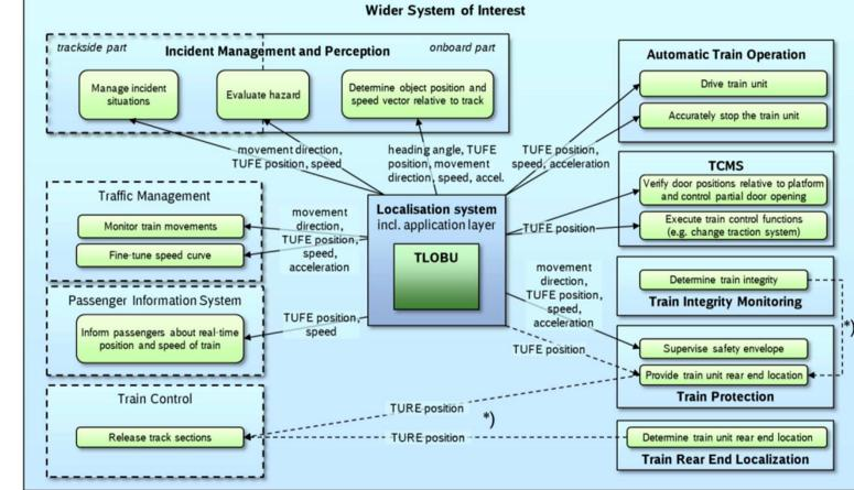
\*) Depending on their type, some trains will determine their rear end indirectly with help of train integrity monitoring and others by a dedicated rear end localization system. The exact distribution of functions for this purpose is outside the scope of CLUG. (see 2.1.5)
