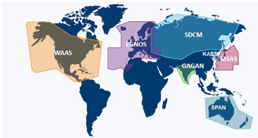
Figure 1: Existing and planned SBAS EGNOS (cf "EGNOS Safety of Life (SoL) Service Definition Document")
